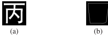
Fig. 3. The effect of convex hull: (a) a Chinese character (b) corresponding convex hull
